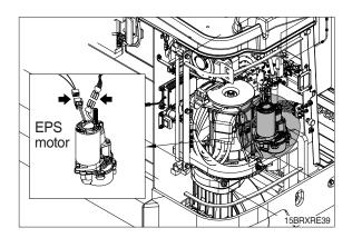
④ Loosen the bolt and remove the EPS motor.
