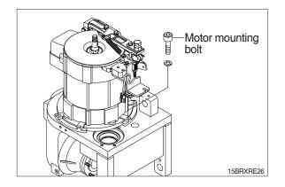
(8) Remove the driving unit mounting bolt to lift with the eye bolt on the motor mounting tab to remove the driving unit.
