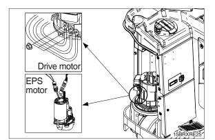
⑤ Remove the bolt connecting the motor and the driving unit.
