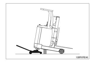
Remove the wheel nut attaching the driving wheel, and take out the driving wheel.
