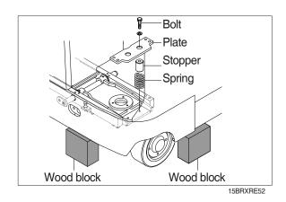
(6) Lift the caster suspension link with a lever.
