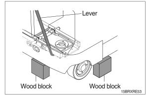
(7) Loosen the bolt and pull the connection pin from the caster suspension link for removal.
